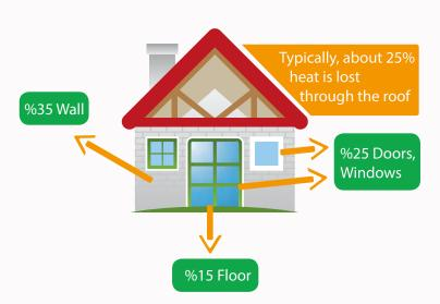
But the cost of insulating the roof is usually much lower than the cost of solid wall insulation, so it is often more cost-effective to do the roof first.
